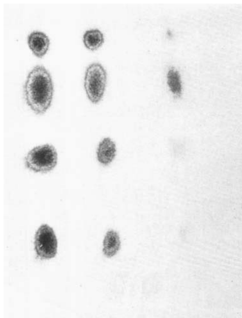
Fig. 1.—Representative separation of acid mixture at different concentration levels: solvent, propanol-formic acid-water (8:1:1); acids in order of increasing R_f value, tartaric, malic, succinic, and mandelic; acid concentrations, from left to right, 50, 25, and 10 mcg. of each component.
